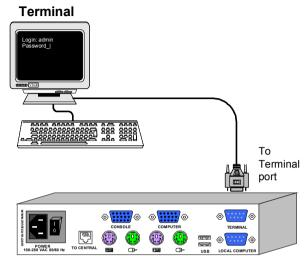
Figure 15 Connecting the RS232 terminal
